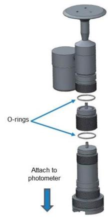
8. Attach column to Photometer inside Enclosure.
