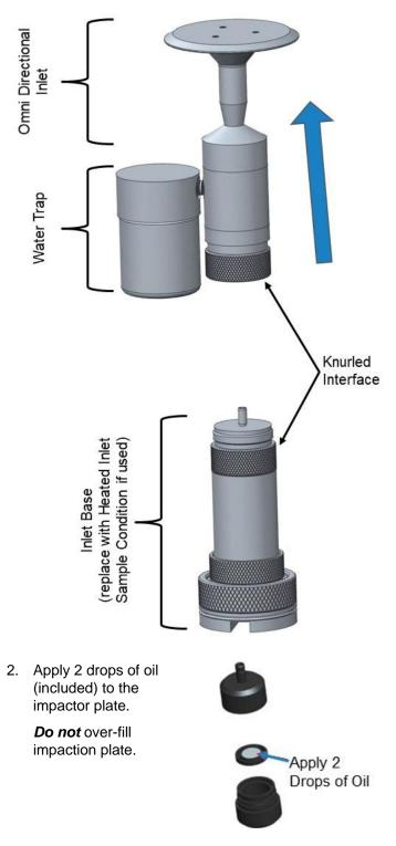
3. Screw (hand-tighten) impactor back together.
