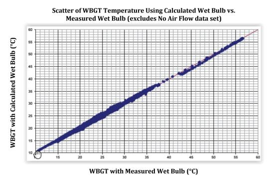
**Figure 4: WBGT measurements (excludes No Air Flow data set)** WBGT temperatures with a natural wet bulb and a waterless wet bulb.
