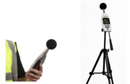
Figure 4-7: Measurement positioning and tripod mount
