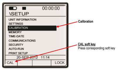
Figure 4-2: Calibration soft key selection
