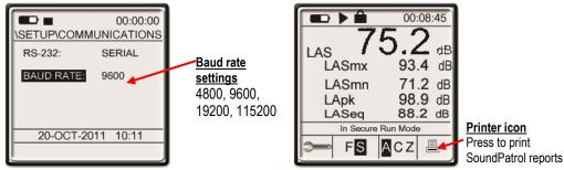
Figure 4-15: Baud rate setup and print icon
