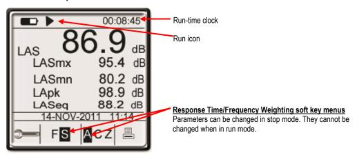
Figure 4-8: Main/multi- measurement screen in Run mode
