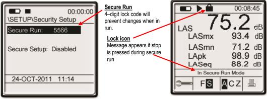
Figure 3-9: Secure run and measurement screen
