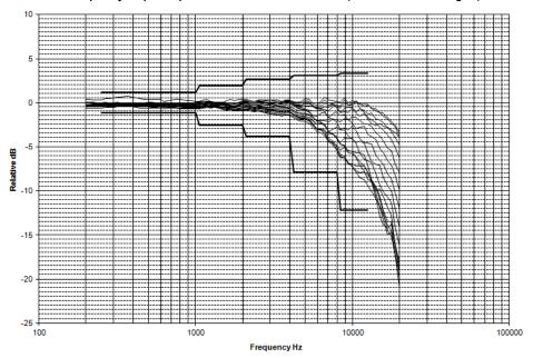
Directional frequency response positioned toward noise source (0°-150° incidence angles)
