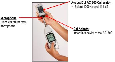
Figure 4-1: SE-400 Series and calibrating
