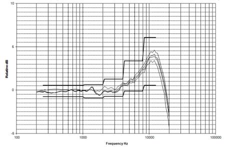
Directional frequency response positioned side toward noise source (0°-90° incidence angles)
