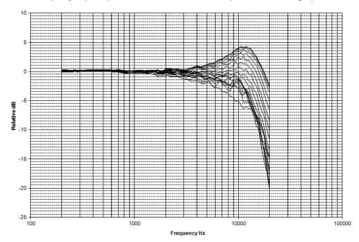
BK4936 microphone with RICR and windscreen back facing Tolerance: IEC 61672 class 1 Directional frequency response positioned back toward noise source (0°-30°incidence angles)
