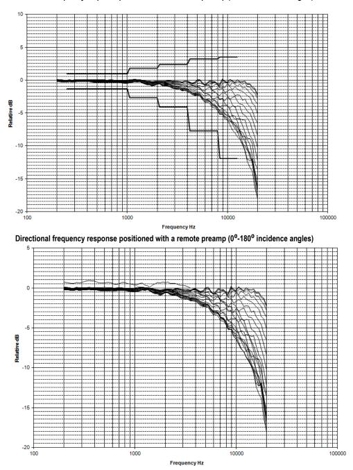
Directional frequency response positioned with a remote preamp (0<sup>0</sup>-150<sup>0</sup> incidence angles)
