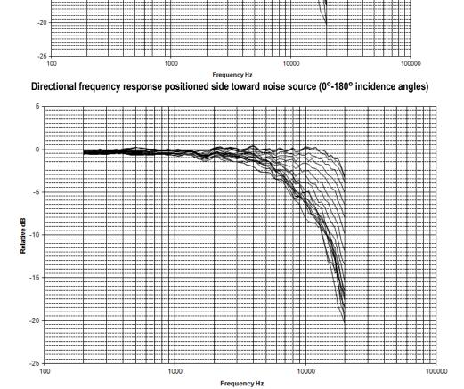
Directional frequency response positioned side toward noise source (0°-150° incidence angles)
