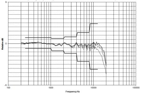
Directional frequency response positioned back-side toward noise source (0°-90° incidence angles)
