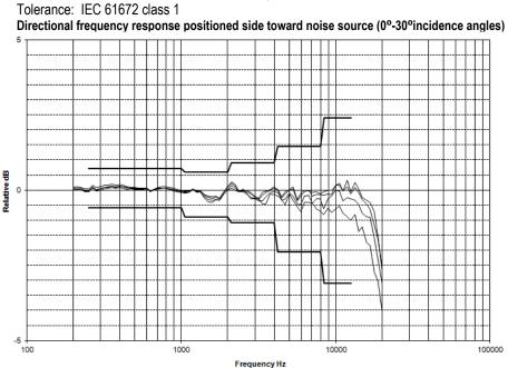
Directional frequency response positioned side toward noise source (0°-90° incidence angles)
