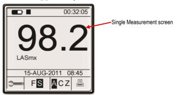
Figure 4-9: Single measurement screen in stop mode
