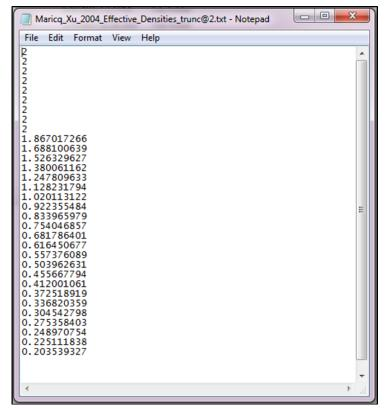
Figure 3: An example text file containing a soot density vector. This text file is loaded into the EEPS software.
