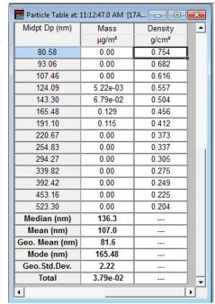
Figure 4: Before and after images of the Particle Table, when updating density values. All non-zero values in the columns for Mass and Density have changed.
