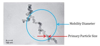
Figure 1: A transmission electron microscope (TEM) image of a soot particle, which is an aggregate of many smaller spherical "primary" particles. The blue circle represents the electrical mobility diameter of the (aggregate) particle.
