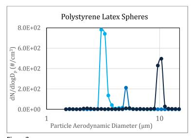
Figure 2 Size distributions of 3  $\mu m$  , 5  $\mu m$  , and 10  $\mu m$  polystyrene latex spheres (PSL) aerosolized by the FMAG
