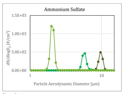
**Figure 3**Size distributions of ammonium sulfate particles generated by the FMAG
