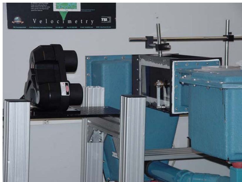
Figure 1: V3V camera probe mounted to take data on the water channel.
