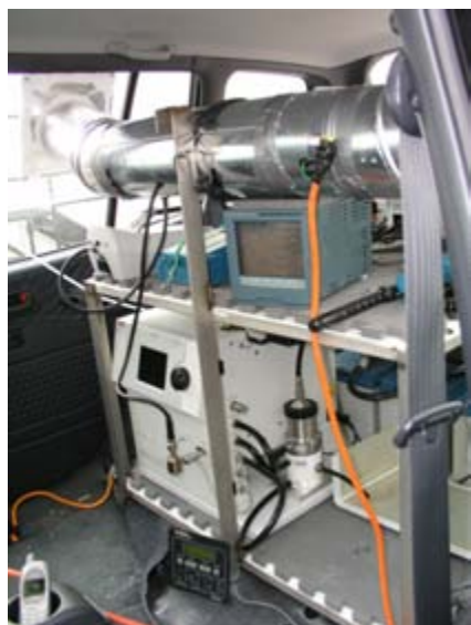
The platform, including duct work, power supplies, and computers for data logging, was jammed into the passenger and luggage compartments, leaving barely enough room for a driver and operator. Photo: Dane Westerdahl
