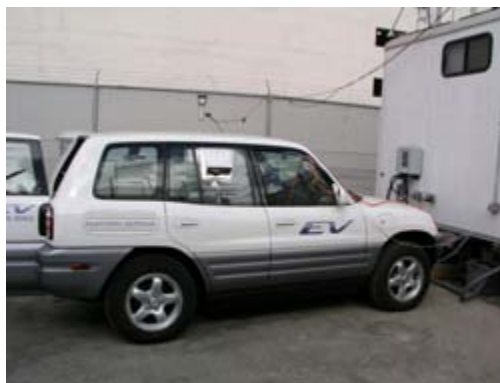
The mobile air-monitoring platform used by California researchers to monitor inside freeway traffic was installed in a Toyota RAV4 electric vehicle. This mobile laboratory provided exciting new data about aerosols in and around high-traffic areas. Photo: Dane Westerdahl
