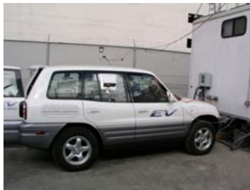
The mobile air-monitoring platform used by California researchers to monitor inside freeway traffic was installed in a Toyota RAV4 electric vehicle. This mobile laboratory provided exciting new data about aerosols in and around high-traffic areas. Photo: Dane Westerdahl
