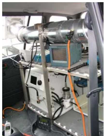
The platform, including duct work, power supplies, and computers for data logging, was jammed into the passenger and luggage compartments, leaving barely enough room for a driver and operator. Photo: Dane Westerdahl
