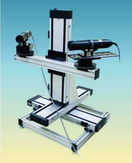
TR260 and TR160 Probes mounted on a traverse
