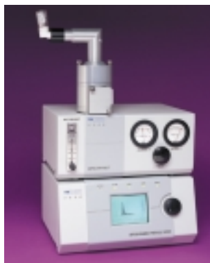
The Model 3306 with MDI throat installed is shown at left atop the Model 3321 APS spectrometer. The spectrometer is sold separately.
