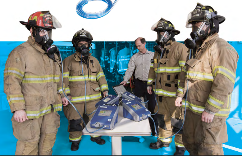
Use the PortaCount Pro Respirator Fit Tester Model 8030 to fit test SCBA masks and CBRN gas masks, and PortaCount Pro+ Fit Tester Model 8038 to fit test SCBA masks, CBRN gas masks and N95 disposable respirators.
