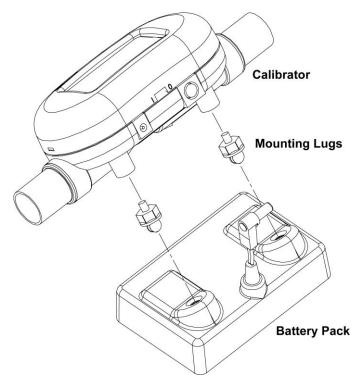
Figure 2-1 Calibrator Assembly
