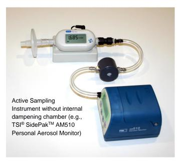
Figure 2-3 Typical Dampening Module Set Up
