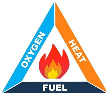
A fire is prevented by “eliminating a side of the fire tetrahedron.” Intrinsic Safety design prevents explosions by eliminating the source of ignition. All components are designed to ensure no heat or sparks above the rated temperature will occur that could ignite gases or vapors.
