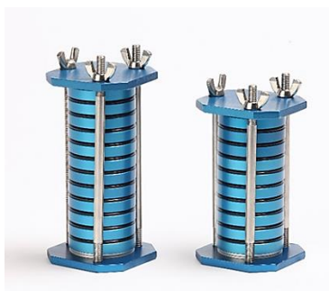
Figure 5: Impaction Plates & Filter Holder.
