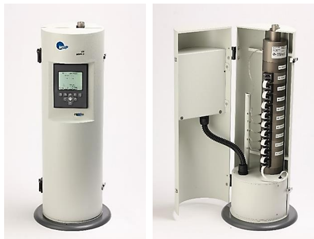
Figure 1: 120R MOUDI II Impactor: exterior (left) and interior (right)
