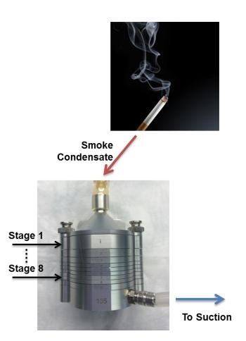
TSI offers a cascade impactor, the Model 135 Mini-MOUDI<sup>™</sup> impactor, which enables separation of smoke aerosol by particle size. The Mini-MOUDI impactor has a small device volume and is designed to handle small flow rates (2 liters per minute or smaller), which match well with the typical smoking puff topographies.
