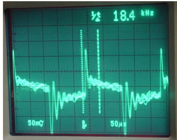
Figure 8. Signal from a film sensor, but time base is too long (50us). Please reduce the time base to 5us.
