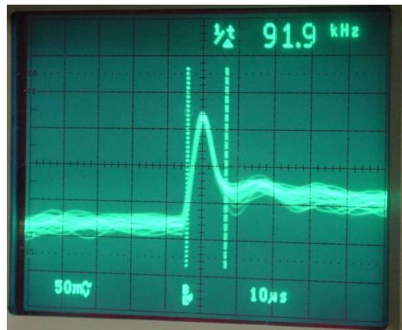
Figure 10. Signal from a film sensor, with acceptable oscillation.
