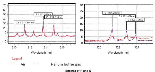
Repeat analysis using a TSI LIBS Desktop Analyzer shows quite acceptable repeatability and accuracy in direct measurement of sulfur and phosphorous in fertilizers. The analysis time in these measurements is less than 20 seconds offering the user substantial benefits in using the TSI LIBS Desktop Analyzer as a process control and optimization tool.
