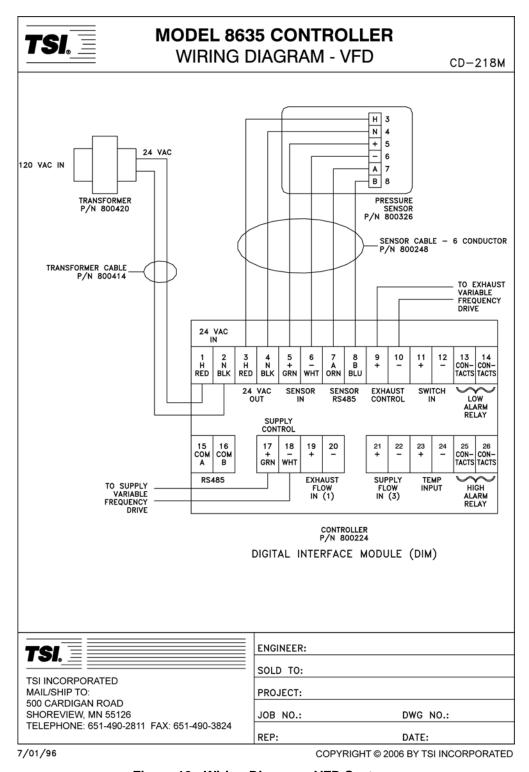
Figure 12: Wiring Diagram - VFD Systems
