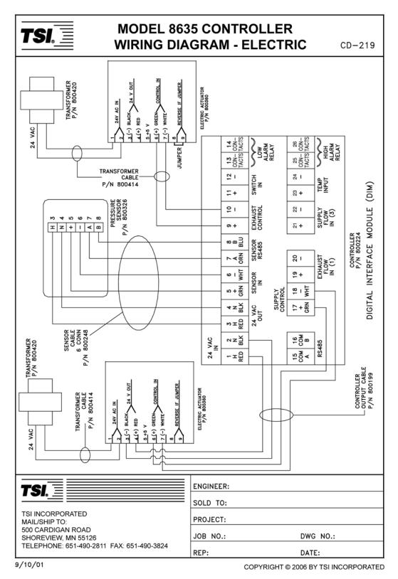
Figure 10: Wiring Diagram - Damper System with Electric Actuator
