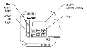
Figure 3: SUREFLOW Operator Panel - Open
