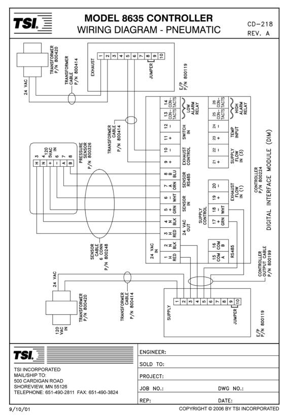
Figure 11: Wiring Diagram - Damper System with Pneumatic Actuator
