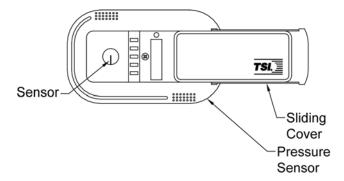
Figure 6: Pressure sensor door slid open
