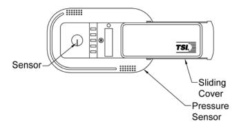
Figure 7: Pressure sensor door slid open
