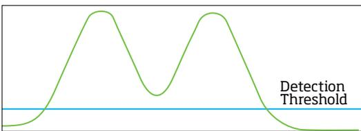
above the threshold and two crests are detected. The time-of-flight between the two crests is recorded and the events are included in the concentration calculations.
