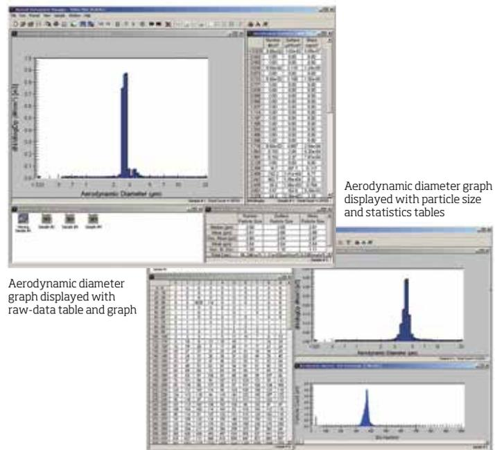
Aerodynamic diameter graph displayed with raw-data table and graph
