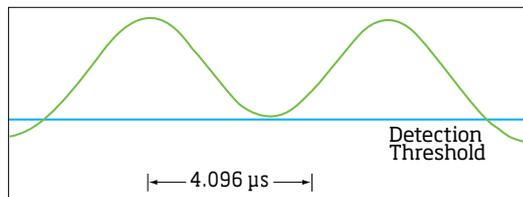
The signal remains above the threshold until it moves outside the timer range, and only one crest is detected. A type 4 event is normally caused by large or recirculating particles. Again, the event is logged, but no time-of-flight is recorded.
