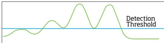
Although the signal stays above the threshold, three or more crests are detected. Events of this type are logged but not recorded for concentration or time-of-flight.
