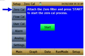
Run **Zero Cal** the first time the instrument is used and repeat prior to every use. Zero Cal requires that the zero filter be attached prior to running. Zero Cal must also be performed if the unit is reading negative concentrations. It is not possible for the DustTrak monitor to read negative concentrations. Negative concentrations are a symptom of zero drift.
