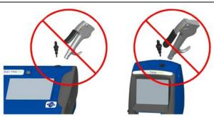
Figure 4-3: DO NOT Blow into Instrument
