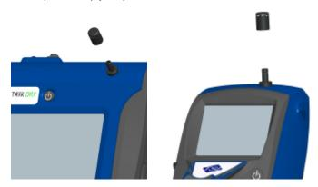
Figure 2-6: Putting on Inlet Cap
