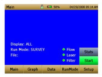
Using a stylus or fingertip, touch the "buttons" on the screen to activate different menus.
