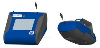
Figure 4-2: Unscrew Inlet Nozzle
