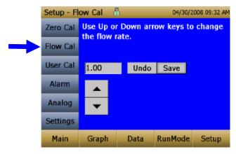
6. Conduct a preflow calibration on the DustTrak monitor using the same kind of sample media you will sample with. Now, attach the sample media you intend to sample with and start sampling aerosol for the desired time. After the desired run time, stop the sampling. Remove the
