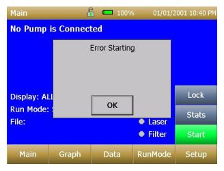
3. If the pump is **not** connected while attempting to perform a Zero Cal, an error appears on the Setup screen.
