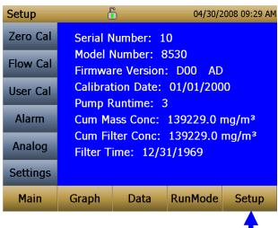
Pressing **Setup** activates the Setup Menu touchscreen buttons along the left edge of the screen. Setup is not accessible when the instrument is sampling.
