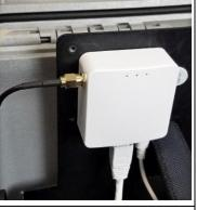
12. Connect the USB cable and RJ45 cable to the DustTrak instrument.
