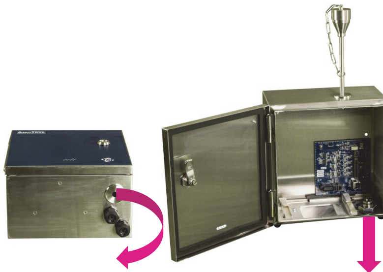
Figure 3. HEPA Filtered sampled air exhausts at the base of the unit, away from the critical work area. The right hand image shows the enclosure with the optics and pump chassis removed.
