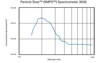
DES test aerosol produced by the model 3079A, measured with TSI's series Scanning Mobility Operation
