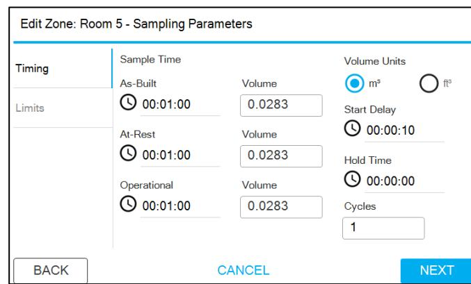
The 'Edit Zone: Room 5 - Sampling Parameters' screen. It shows 'Timing' and 'Limits' tabs. Under 'Timing', 'Sample Time' is set to 'As-Built' with a value of '00:01:00'. 'Volume' is set to '0.0283' and 'Volume Units' is set to 'm³'. Under 'Limits', 'At-Rest' and 'Operational' are both set to '00:01:00'. 'Volume' is set to '0.0283' for both. 'Start Delay' is '00:00:10', 'Hold Time' is '00:00:00', and 'Cycles' is '1'. At the bottom are 'BACK', 'CANCEL', and 'NEXT' buttons.
