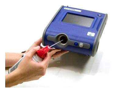
Reinsert the alcohol cartridge. Turn the PortaCount Pro Respirator Fit Tester on. Perform the Daily Checks. If the problem persists, try Procedure B.
