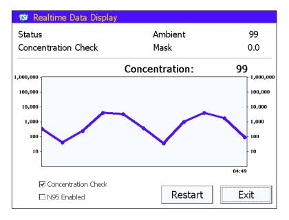
In this mode, the PortaCount Pro fit tester continuously measures the particle concentration through the ambient inlet port allowing the user to easily check ambient concentration in preparation for testing.
