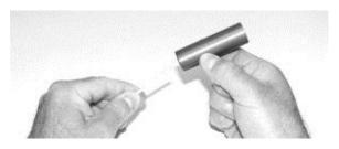
3. Examine the white Alcohol Wick. Discard wicks that are severely discolored or physically damaged. Some light brownish-yellow discoloration of the wick is normal.
