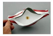
*For flat "duckbill" style respirators*, install the probe near the outer edge of the *bottom panel* where it cannot be blocked by the person's chin.
