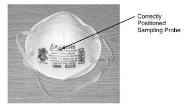
Note Once a sampling probe is installed into a disposable mask, the mask cannot be used for respiratory protection. **Probed masks are to be used for quantitative fit testing only.** Discard each probed disposable mask after a fit test is completed.
