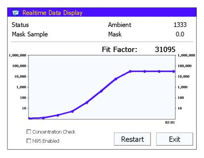
The PortaCount Pro Respirator Fit Tester takes an ambient concentration reading and stores the value. Next it purges the mask and then begins continuous monitoring of the mask concentration.
