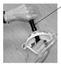
Push the Tools Together to Fasten the Probes 9. Inspect the sampling probe to be sure it is not plugged. Try to rotate the probe with your fingers. If it moves freely, use the probe insertion tool kit to press the push nut firmly onto the sampling probe and pinch the mask material more tightly.
