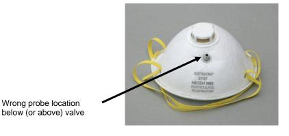
*For respirators with an outer mesh*, install the probe normally as if the mesh was not present. The sampling probe and push nut will seal properly right through the mesh.
