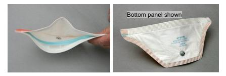
*For respirators with center-mounted exhalation valves*, install the probe to the left or right of the valve. Do **not** install the probe above or below the valve because this risks having the probe blocked by the person's nose or chin.
