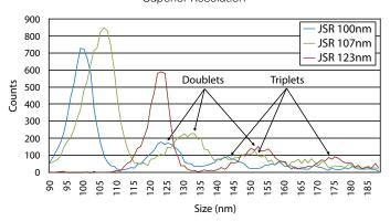
Typical resolution is within 2.5% of the particle diameter at 0.1 µm. The model 3340A can differentiate between 100 nm and 107 nm PSL!
