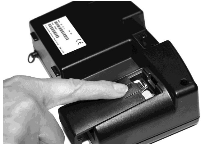
Figure 5 Battery Cover Removal
