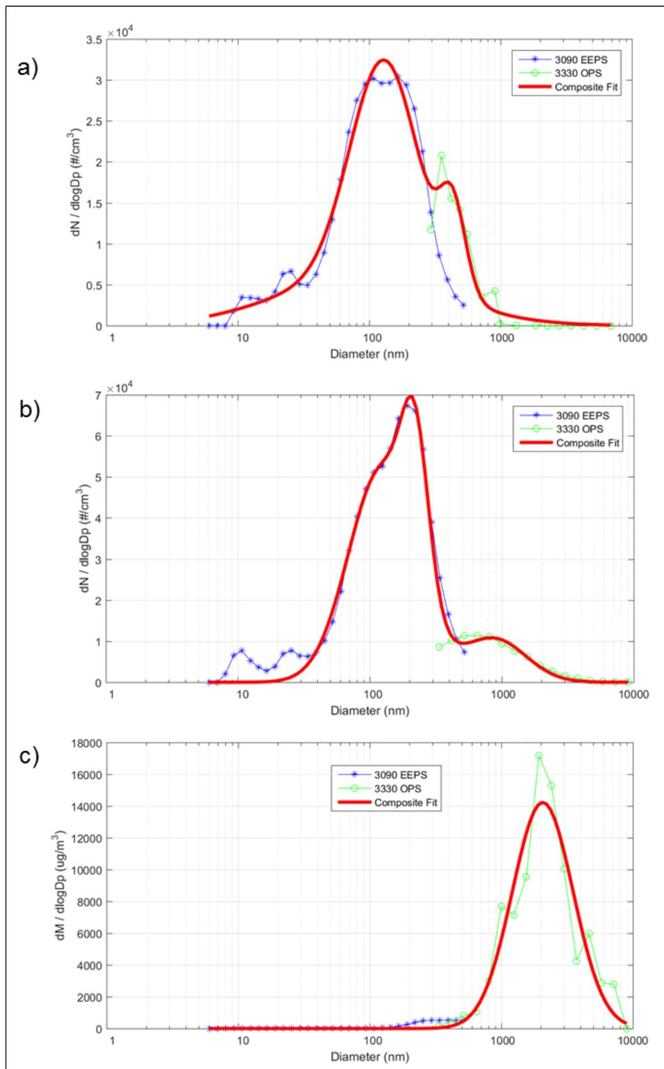
**Figure 4, a-c: Particle number concentrations from brake events with low (a) and high (b) energy; calculated particle mass concentration (using a density of  $1 \text{ g m}^{-3}$ ) from the brake event shown in Panel c (same scan as b).**
