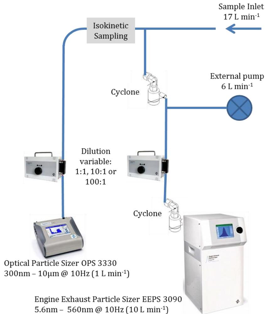
Figure 1: Schematic of the Wide Range Fast Sizer System with EEPS Spectrometer and OPS
