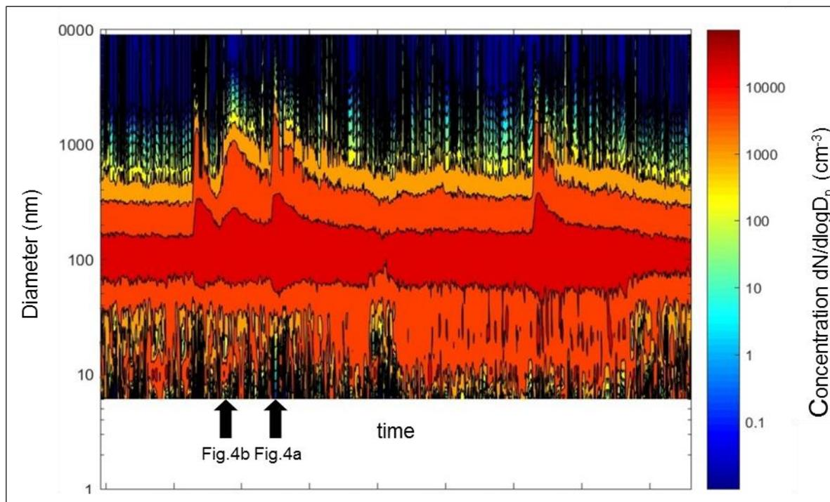
Figure 5: Time series of merged size distributions with a time resolution of 10 Hz for several braking events. The plot shows approximately 2.5 minutes of data for the size range of 6 nm – 10  $\mu\text{m}$ . The number concentration is shown in the color scale at right. The arrows indicate the time of selected scan shown in Figure 4.
