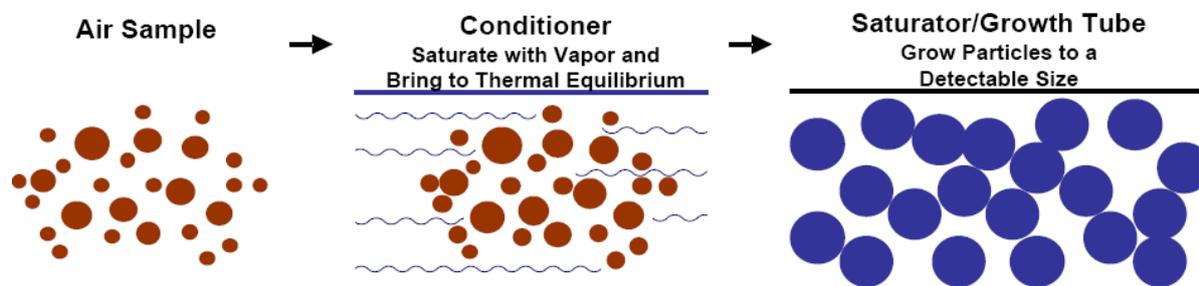
Figure 1: Continuous, laminar flow condensation particle counter (CPC) operation.
