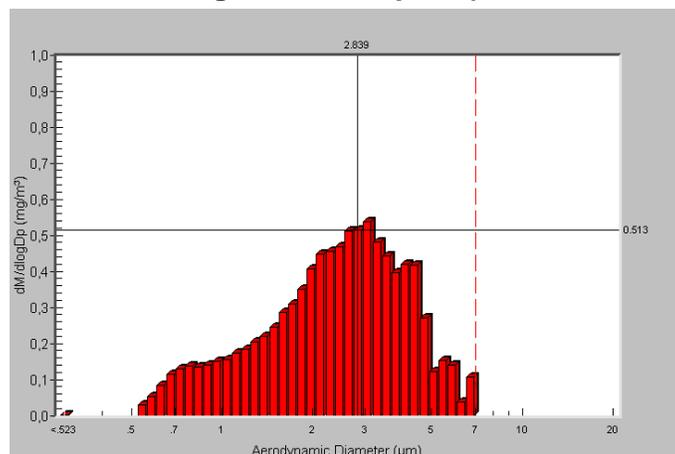
The aerodynamic size distribution of the suspension pMDI again is a non-Gaussian one that indicates two modes. The 3D-plot reveals this even more clearly: one mode is of a very narrow, submicrometer aerodynamic size with a wide light scattering range, while the other mode ranges from 1 to ~6  $\mu\text{m}$  in aerodynamic size but only a small scatter around an intensity of about 10.
