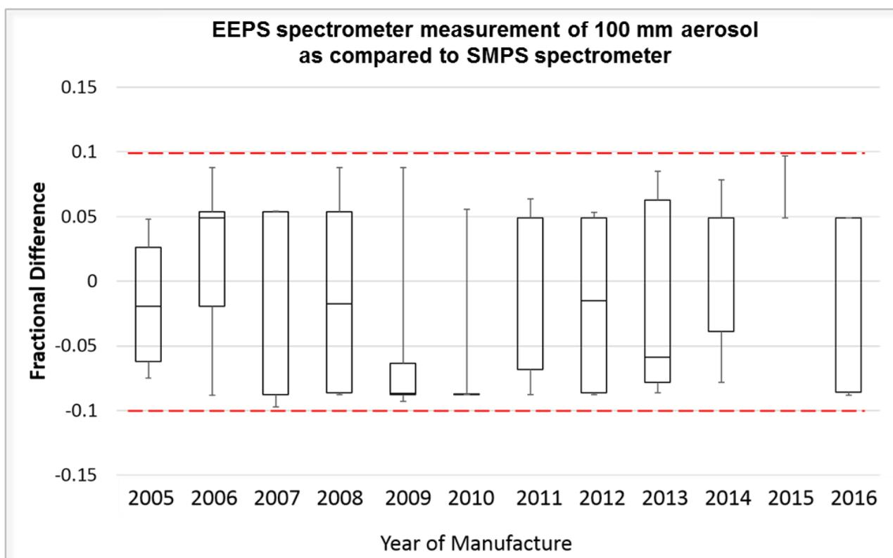
**Figure 1:** EEPS instruments' measurement of 100 nm classified aerosol, compared to SMPS spectrometer measurement of the same aerosol, grouped by year of manufacture. The oddly shaped plot for 2015 is due to the fact that 92% of EEPS instruments manufactured that year deviated from SMPS measurements by the same value, ~ 5%. The dashed lines represent  $\pm 10\%$ , TSI's internal requirement for EEPS-SMPS agreement.
