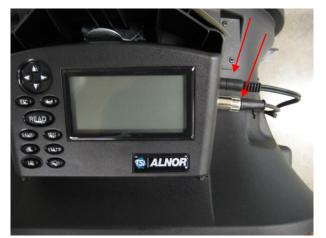
2. Pinch strain relief bushing and push through the base hole.
