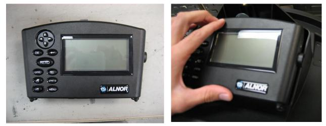
7. Locate custom cable and thermister probe cord and insert them into their respective ports in the micromanometer.
