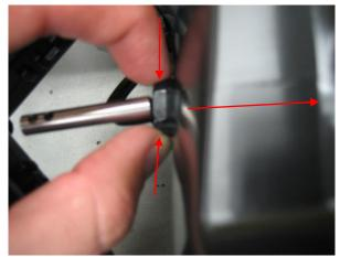
3. Open the strain relief bushing and remove the thermister probe cord only.
