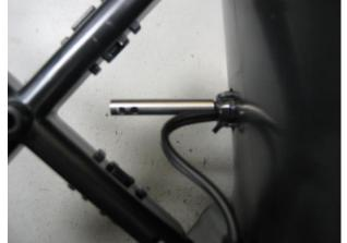
6. Locate the micromanometer and insert into the micromanometer port in the base. Snap in to secure.
