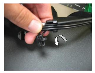
4. Locate new thermister probe and insert it into the strain relief bushing.
