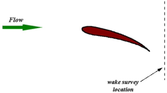
The free stream velocity of the air flow was about 9.5 m/sec. The flow was seeded using water droplets. The LDV system was operated in the coincidence mode to measure all three components of velocity simultaneously.
