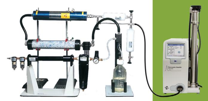
This 3940A system is shown ready to calibrate a TSI® Electrostatic Classifier 3082. Ask your TSI® representative about additional components needed for your particular application.
