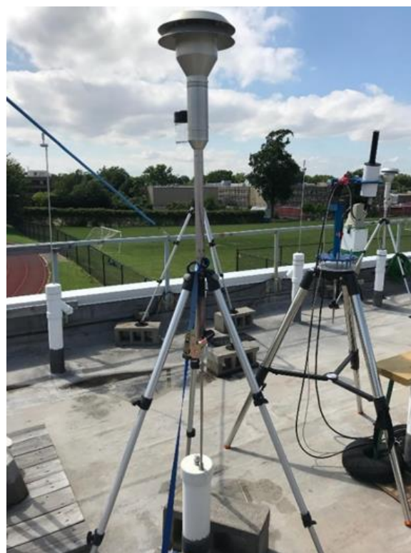
Figure 1: Sampling inlet for QCM-MOUDI™ impactor.
