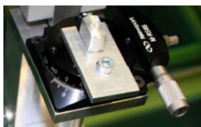
Fig. 3. Rotary table for angle adjustment
