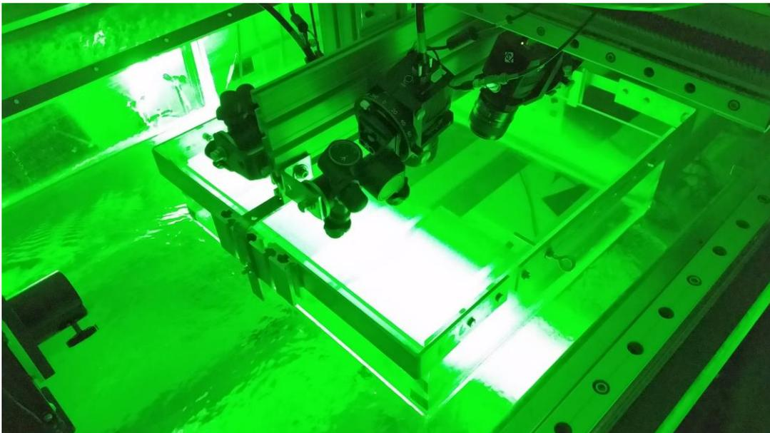
**Fig. 1.** Experimental setup showing the cameras viewing the boundary layer flow through the glass box placed at the surface, and the laser illuminating the measurement region.
