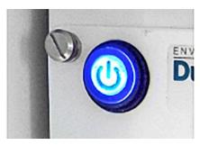
11. The LED on the modem will blink while the modem searches for a suitable network. If the LED stops blinking and is solid blue, a network has been found and proper communication with Environet™ should be possible. If the LED changes to solid yellow, the modem has not found a network. A power cycle may resolve the issue or the unit may need to be moved to a different location where signal strength is improved.
