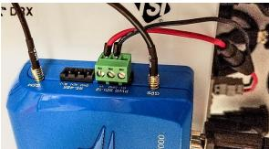
10. Plug the AC/DC power supply into an AC power source. Instrument and modem should power on.
