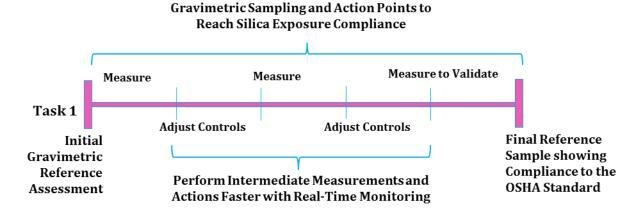
It is important to note that the use of real-time instruments will not totally replace the need for gravimetric sampling; however, real-time monitoring can minimize the number of gravimetric samples taken. As stated earlier, gravimetric sampling is needed as a reference measurement at the beginning and again at the end of an initial exposure assessment as well as when completing follow-up assessments in order to prove compliance.
