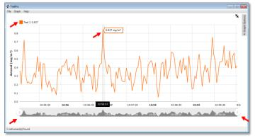
Data logged with real-time instruments help employers get a better understanding of silica exposure in real time to gain insights into the relationship between a worker's activity and silica exposure levels during an entire shift—without having to wait for lab results.
