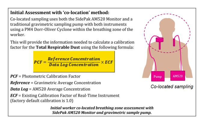
**Gravimetric Sample Pump:** The gravimetric sample is collected via a sample pump with a collection filter that is sent to an accredited laboratory for analysis. The lab will provide a report of the analysis that contains the following information:
