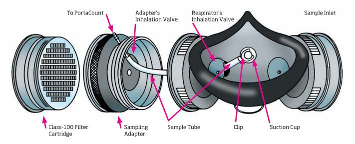
Exploded view showing how a typical fit test adapter is installed onto a respirator. Individual adapters differ in design.
