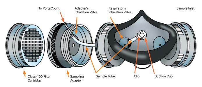
Exploded view showing how a typical fit test adapter is installed onto a respirator. Individual adapters differ in design.
