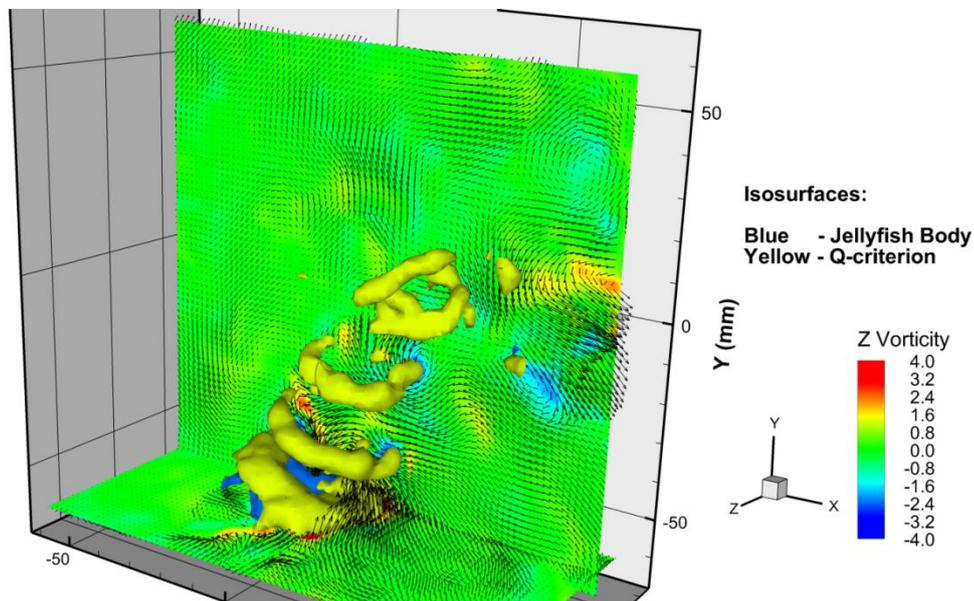
**Fig. 2.** Single, instantaneous velocity field of the jellyfish wake. The body of the jellyfish is seen in the blue isosurface. Q-criterion, representing vortex cores, is visualized in yellow isocontours. The color of the planes represents vorticity.
